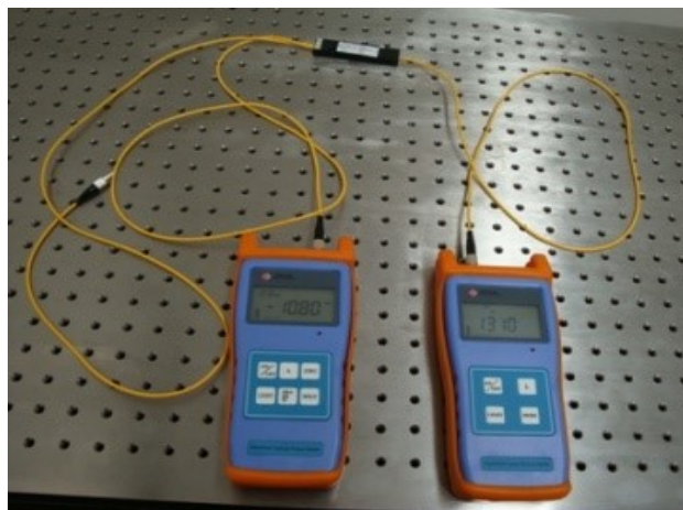
Figure 21 Photo of experimental setup for splitter measurement
