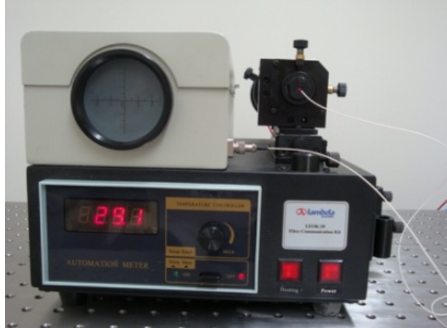
Figure 17 Photo of experimental setup for fiber temperature sensing
