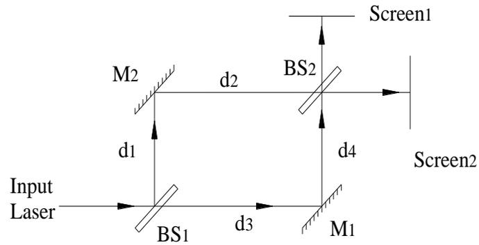
Figure 5-3 Schematic of Mach-Zehnder interferometer
