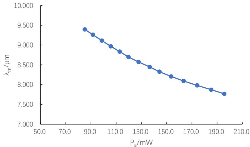
Figure 5. Relationship Between Radiant Power  $P_a$  and Peak Wavelength  $\lambda_m$
