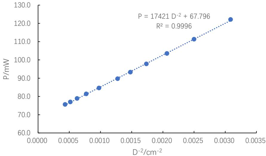
Figure 6 Relationship between the inverse square of distance  $D^{-2}$  and average radiation power  $P$ . The linear fit shows a good degree of linearity. The intercept of the fitted line is 67.796 mW, which is very close to the measured environmental background radiation power  $P_0=69.6$  mW. This indicates that when the distance  $D$  between the blackbody emitter and the thermal imager approaches infinity, the thermal imager receives only the environmental background radiation power.
