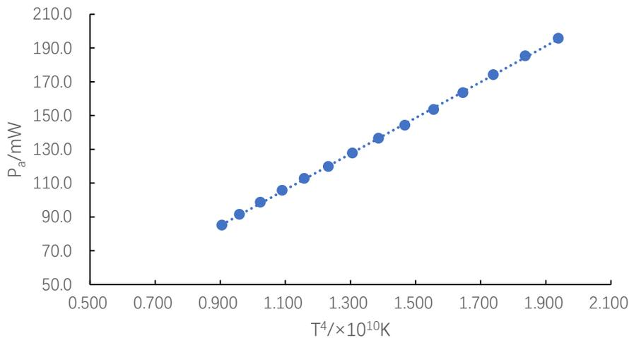
Figure 4. Relationship Graph Between Blackbody Emitter Temperature  $T^4$  and Radiant Power  $P_a$
