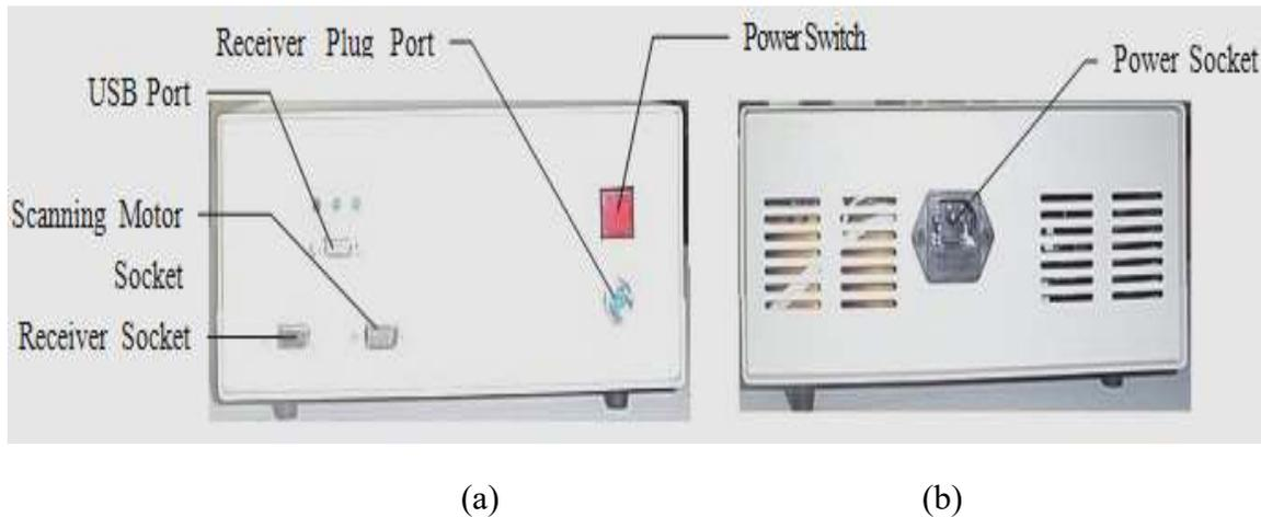
Figure 8 Front (a) and back (b) panel of electrical control box
