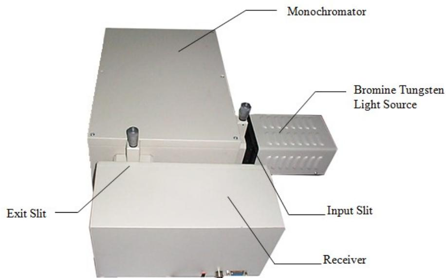
Figure 2 Description of experimental apparatus
