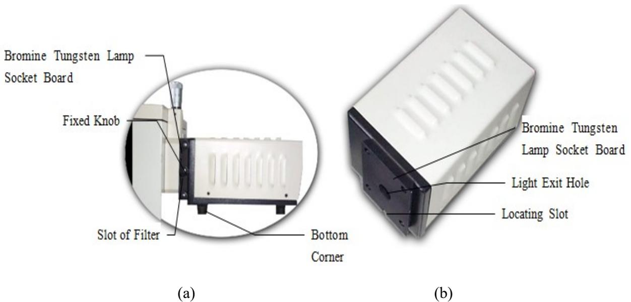
Figure 6 Illustration of Bromine-Tungsten lamp attached to monochromator (a) and description of Bromine-Tungsten lamp
