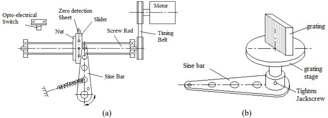
Figure 4 Schematic of scanning mechanism (a) and grating rotation stage (b)
