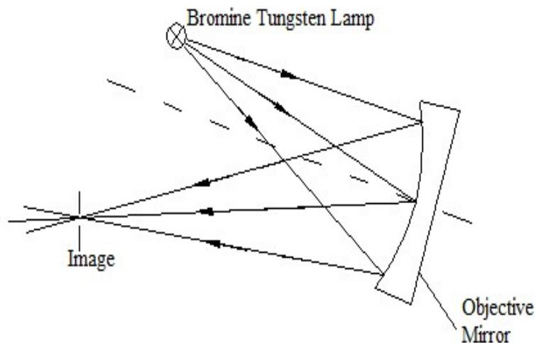
Figure 7 Optical diagram of Bromine-Tungsten light source
