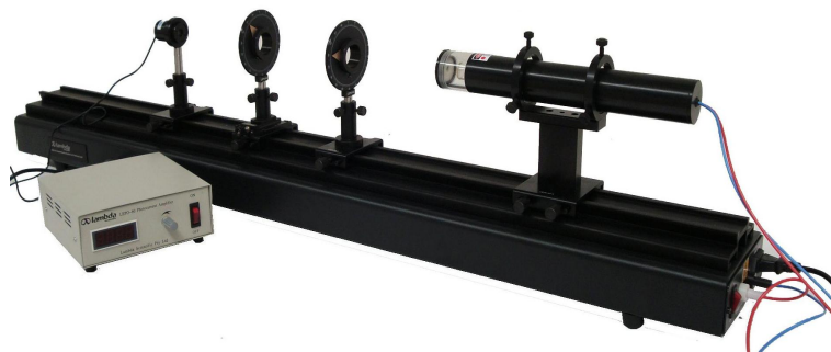
Figure 5 Experimental setup for verification of Malus's Law
