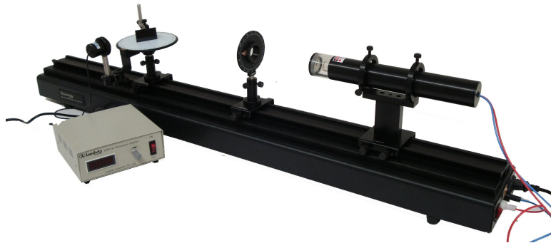
Figure 1 Experimental setup for measurement of Brewster's angle
