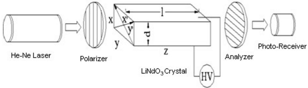
Figure 2 Schematic of transverse electro-optic modulation
