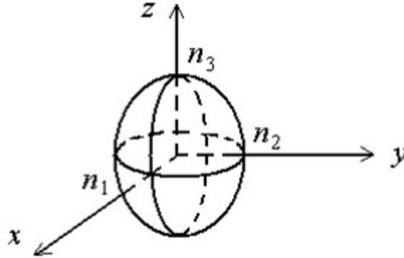
Figure 1 Refractive index ellipsoid in the absence of an electric field
