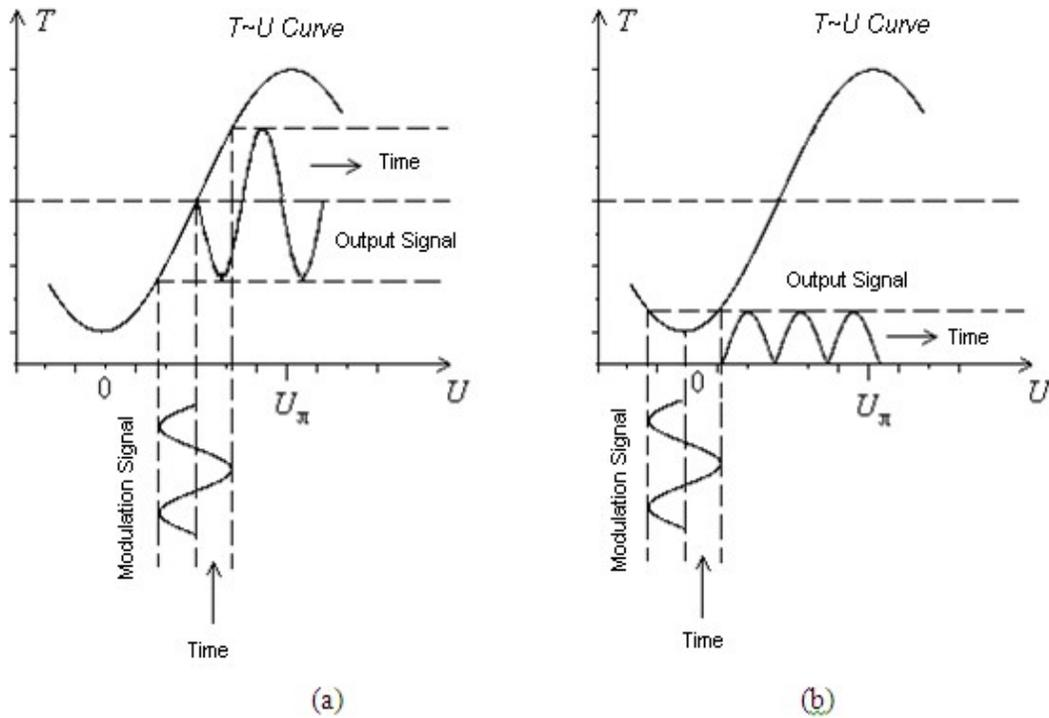
Figure 3 Effect of dc voltage bias on output characteristic of electro-optic crystal
