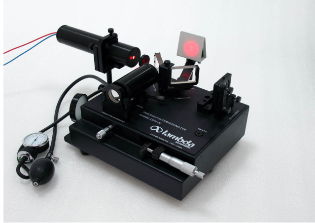
Figure 11 Michelson interferometer with air chamber in optical path
