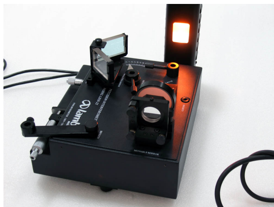
Figure 16 Fabry-Perot interferometer with Sodium lamp as light source
