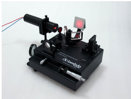
Figure 5 Michelson interferometer with He-Ne laser as light source
