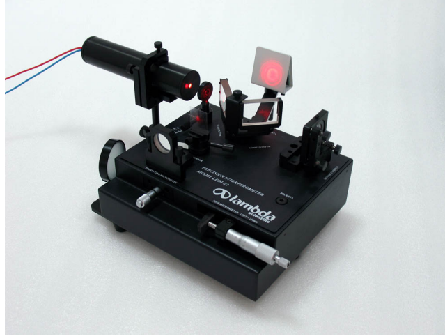
Figure 12 Michelson interferometer with transparent slice in optical path
