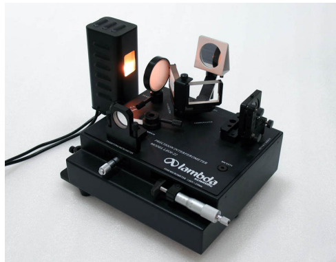
Figure 6 Michelson interferometer with Sodium lamp as light source
