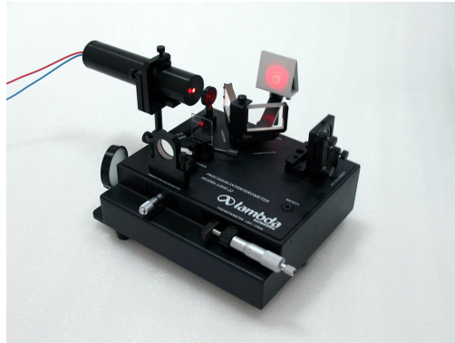
Figure 22 Twyman-Green interferometer configured for checking transparent flat optic
