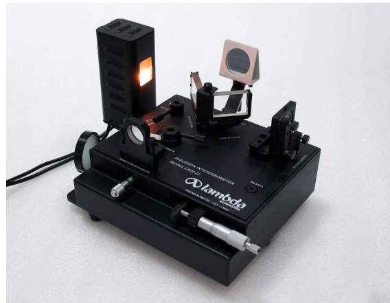
Figure 10 Michelson interferometer with Sodium-Tungsten lamp as light source
