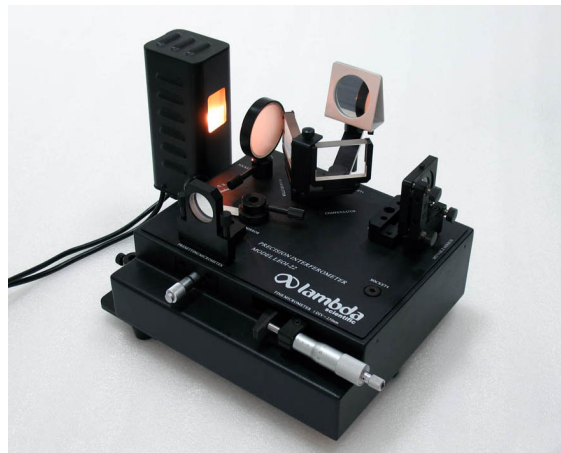
Figure 9 Michelson interferometer with Sodium-Tungsten lamp as light source
