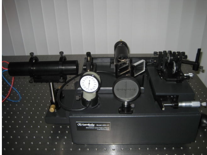
Figure 10 Michelson interferometer with air chamber in optical path
