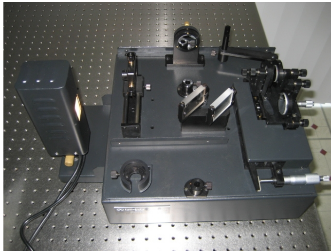
Figure 8 Michelson interferometer with Sodium-Tungsten lamp as light source
