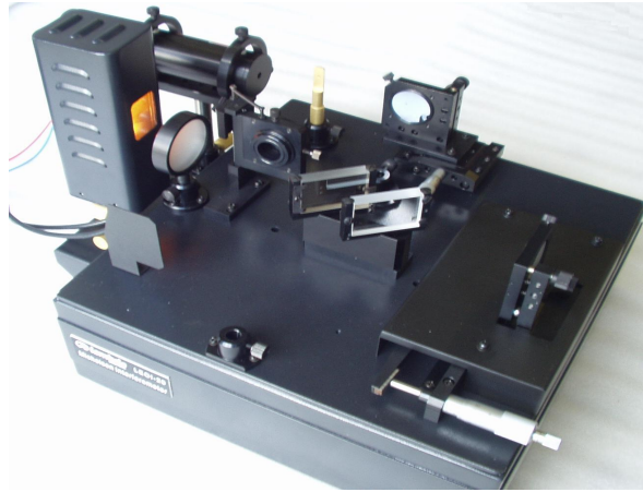
Figure 8 Michelson interferometer with Sodium-Tungsten lamp as light source
