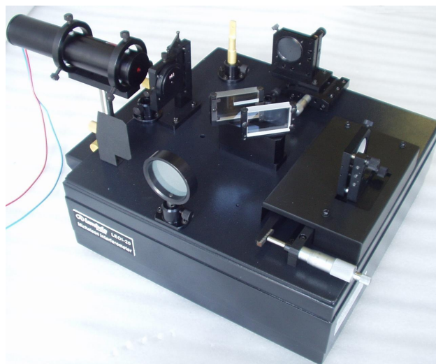
Figure 3 Michelson interferometer with He-Ne laser as light source
