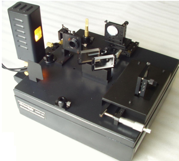
Figure 4 Michelson interferometer with Sodium lamp as light source
