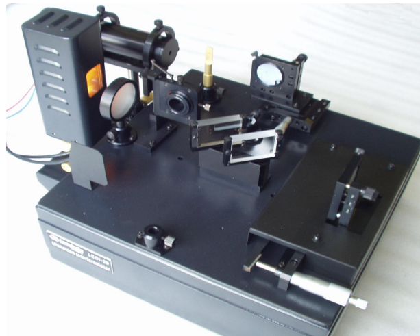
Figure 7 Michelson interferometer with Sodium-Tungsten lamp as light source
