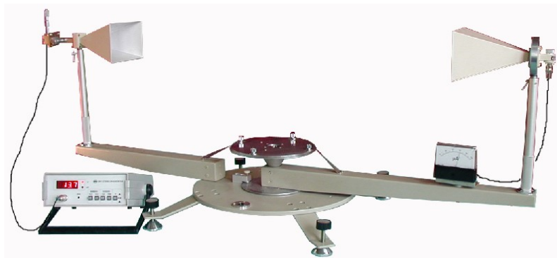
Figure 9 Setup of polarization experiment
