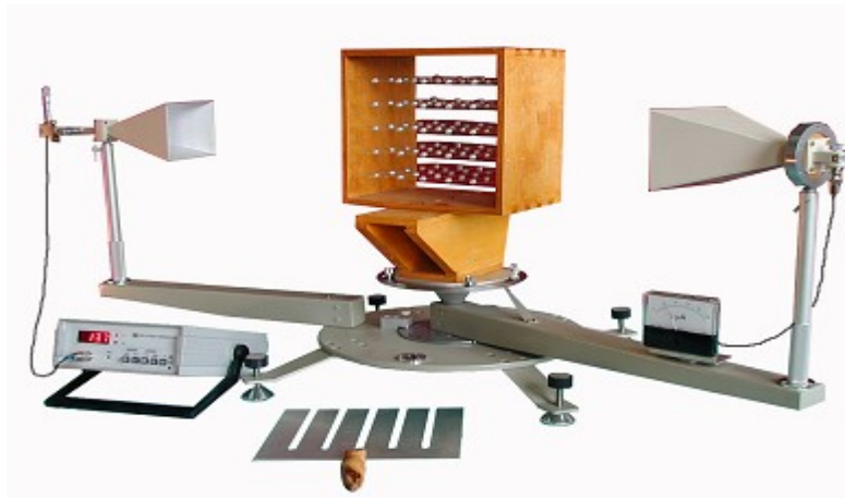
Figure 10 Setup of Bragg diffraction experiment
