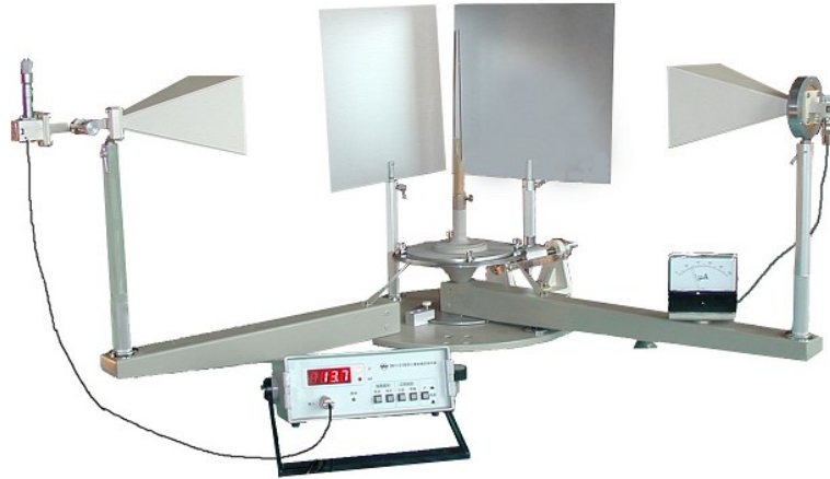
Figure 8 Setup of Michelson Interferometer
