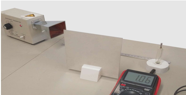
Figure 6 Experimental setup for interference of microwave
