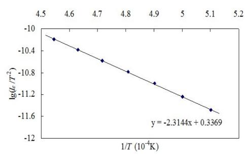
The slope of the fitted line is -23144, calculate the escape potential as 4.59 V using formula (2), and compared with the theoretical value of 4.54 V, leading to a relative error of  $\sim 1.1\%$ .
