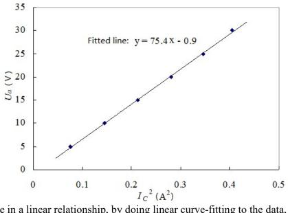
As  $U_a$  and  $I_c^2$  are in a linear relationship, by doing linear curve-fitting to the data, the fitted slope is 75.4. Using formula (11), the charge-mass ratio of electron is calculated as  $1.805 \times 10^{11}$  C/Kg. Compared with the theoretical value of  $1.759 \times 10^{11}$  C/Kg, the relative error is 2.6%.
