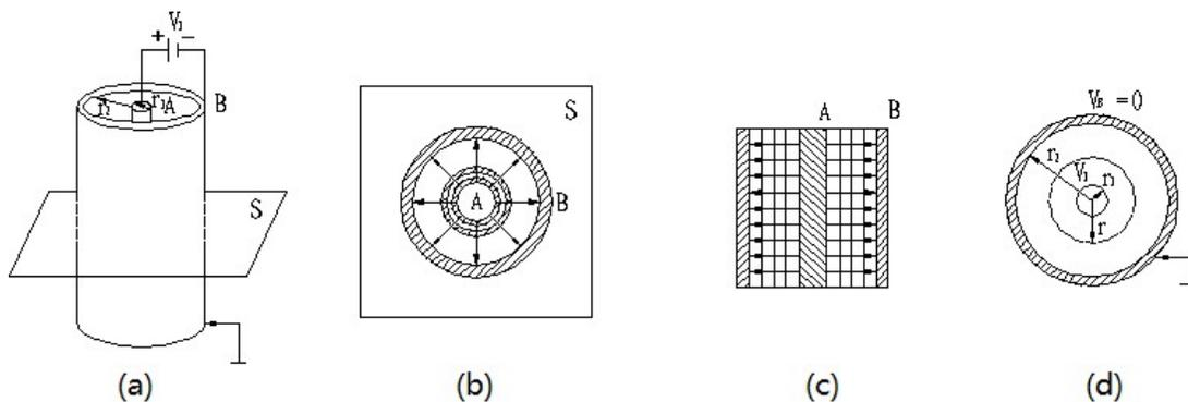
Figure 2 Electric field of a long coaxial electrode: (a) electrode structure, (b) electric line distribution in the perpendicular cross section, (c) electric line distribution in the longitudinal cross section, and (d) schematic for calculation
