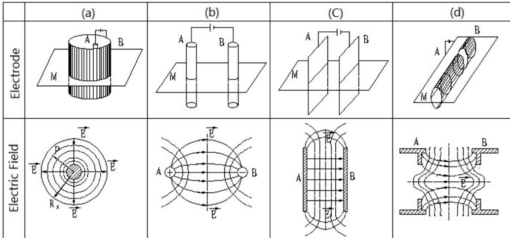
Figure 1 Examples of electrode patterns and corresponding electrostatic field equipotential lines distributions: (a) coaxial cable, (b) parallel-wire, (c) parallel-plane and (d) focusing electrode
