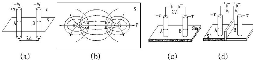
Figure 4 Electric field of a pair of long parallel lines
