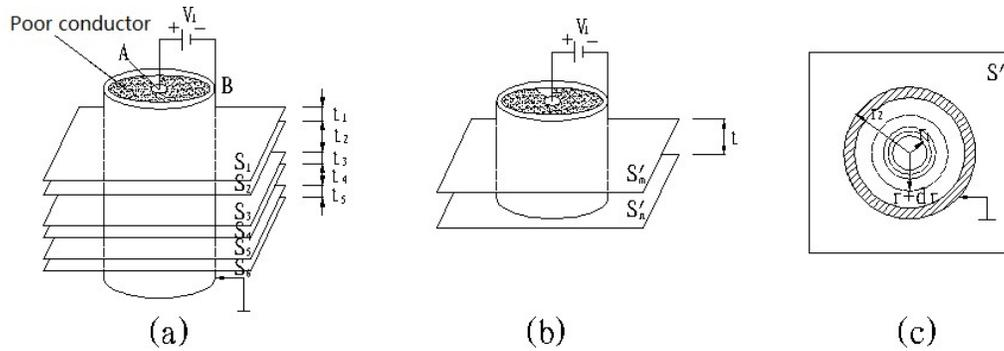
Figure 3 Current field of a long coaxial cable: (a) cable structure, (b) current line distribution in the perpendicular cross section, (c) schematic for calculation
