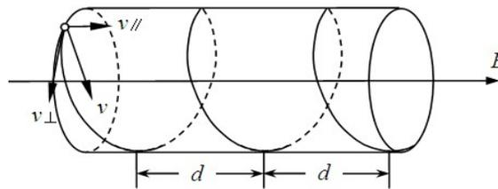
Figure 7 Spiral motion of electron in magnetic field
