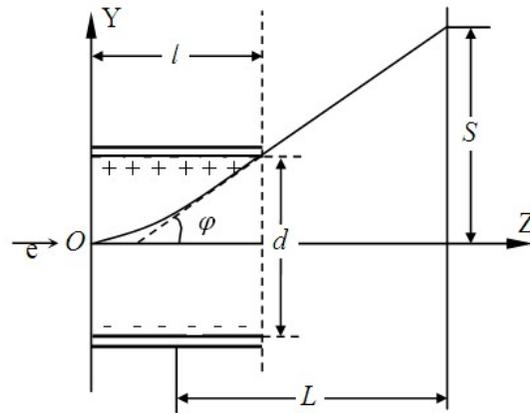
Figure 3 Principle of electric deflection
