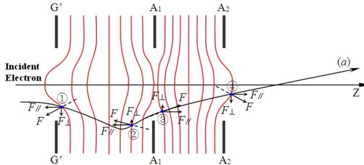
Figure 4 Schematic of electron trajectory by electric focusing
