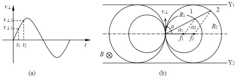
Figure 8 Spiral traces of electrons in AC magnetic field
