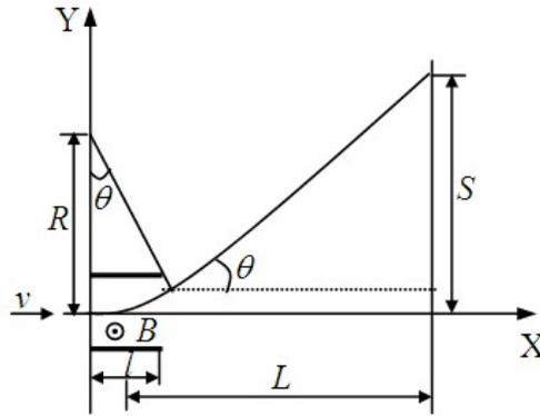
Figure 6 Electron deflection after leaving magnetic field
