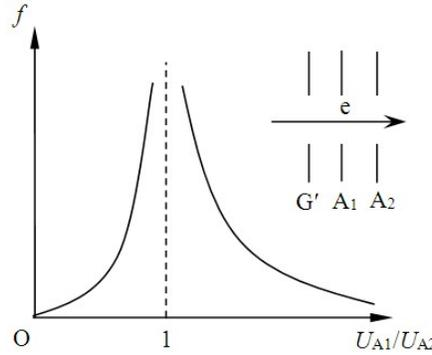
Figure 5  $f \sim U_{A1}/U_{A2}$  curve of CRT
