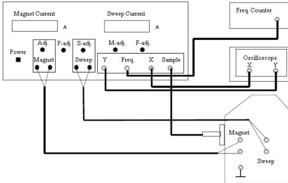
Figure 2 Schematic of NMR system
