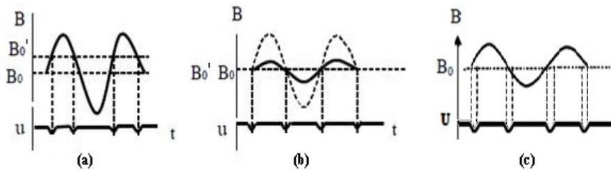
Figure 6 Relationship between resonance absorption signal waveform and magnetic field
