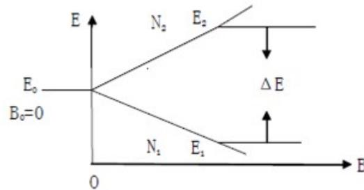
Figure 1 Zeeman splitting of energy level in magnetic field
