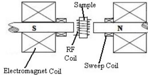
Figure 4 Electromagnet, sweep and RF coils
