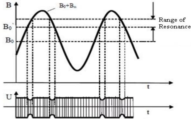
Figure 5 Magnetic field and resonance absorption
