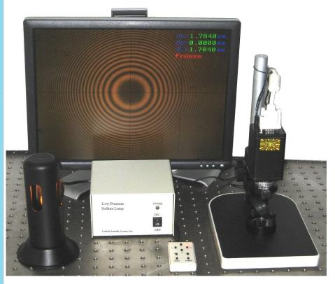
The phenomenon of Newton's rings, named after Isaac Newton, is an interference pattern caused by the reflection of light between two surfaces - a spherical surface and an adjacent flat surface. When viewed with monochromatic light, it appears as a series of concentric, alternating light and dark rings centered at the point of contact between the two surfaces.
