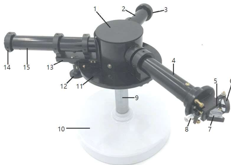
Configuration of Kirchhoff Bunsen spectroscope
