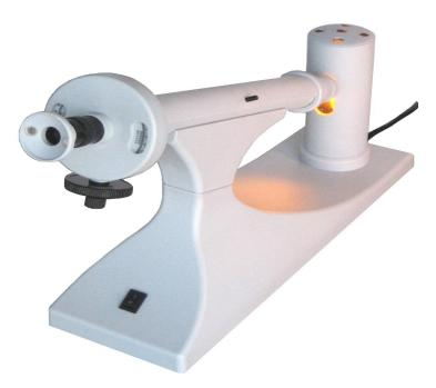
A polarimeter is an instrument to measure the degree of the optical active rotation of a sample, from which the concentration, purity, sugar content, or content of the sample can be determined. It is widely used in sugar refining, pharmaceutical, drug test, food, spices, monosodium glutamate, as well as chemical, oil and other industrial production, scientific research or quality control inspection process.
