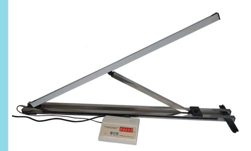
Magnetic damping is an important concept in electromagnetism. The mechanical effect of magnetic damping has very important applications. This experimental apparatus is designed to measure the uniform sliding speed of a magnetic slide on a non-ferromagnetic conductor inclined rail. Through data processing, magnetic damping coefficient and sliding friction coefficient are acquired. This experimental apparatus is related to physics concepts such as mechanics and electromagnetism.
