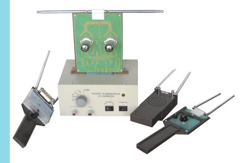
This LEEI-60 experimental apparatus of transmission and reception of electromagnetic waves is designed for teaching electromagnetic oscillation and wave in general physics. It is useful for demonstrating the transmission, reception, modulation, electric resonance, tuning as well as the characteristics of electromagnetic waves. It is an affordable teaching apparatus for physics laboratories in colleges and universities.
