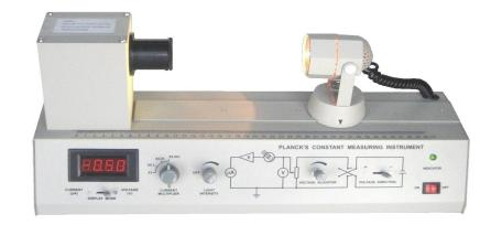
This LEAI-50 Experiment Apparatus of Planck's Constant is used to demonstrate photoelectric effect and calculate Planck's constant according to Einstein's equation of photoelectric effect. It is a cost-effective teaching apparatus for physics laboratories at colleges and universities.
