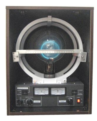
This LEAI-48 Lorentz force demonstrator is useful for testing the electron charge/mass ratio (e/m), also useful for demonstrating the Lorenz force exerted by a magnetic field on moving electrons and the deflection of moving electrons within an electric field. It is an affordable teaching apparatus for physics laboratories in colleges and universities.
