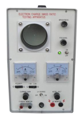
This LEAI-45 experimental apparatus is designed to determine the specific charge of an electron, i.e. charge/mass ratio (e/m), based on the longitudinal magnetic field focusing method. It is an ideal teaching apparatus for physics laboratories at colleges and universities.
