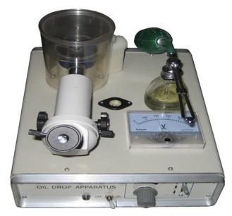
This LEAI-40 apparatus of Millikan oil droplet experiment is designed to verify the quantum nature of electrical charges, measure the elementary charge of an electron, and observe the Brownian motion. Using an optional VGA camera with built-in electronic grid lines, oil drop image can be acquired and displayed in real-time on a LCD monitor for more convenient observation and accurate measurement. It is an ideal physics teaching apparatus for colleges and universities.
