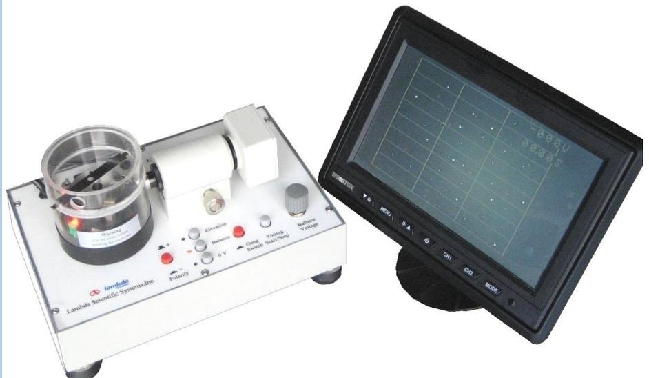
This LEAI-42 apparatus of Millikan's oil drop experiment is the advanced version of the series with CCD image acquisition and monitor display, it is designed to verify the quantum nature of electrical charges, measure the elementary charge of an electron, experiment on the Brownian motion, and verify normal distribution of displacement probability. It is an ideal physics teaching apparatus at colleges and universities.
