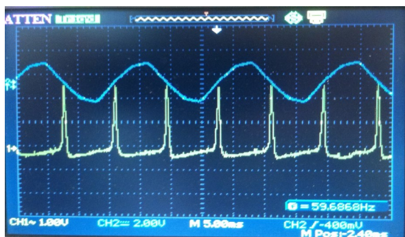
Electron resonance signal on oscilloscope
